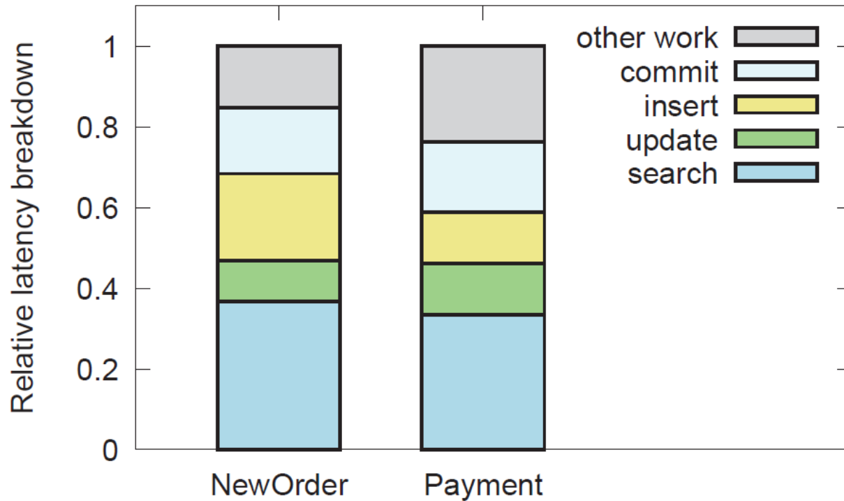
Figure 19: Breakdown of TPC-C-NP-Insert, 224 threads, 224 warehouses, NewOrder and Payment transactions
